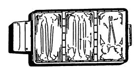
Note: Do not obstruct the small holes at the back of the cassette! The steam and condensate pass through these openings.
